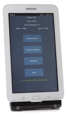
Figure 3: Main Menu of the ALIAS™ tablet control software
