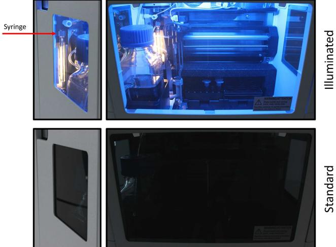
Figure 2: Inside and syringe illumination for air bubble detection in comparison with the ALIAS™ standard model.
